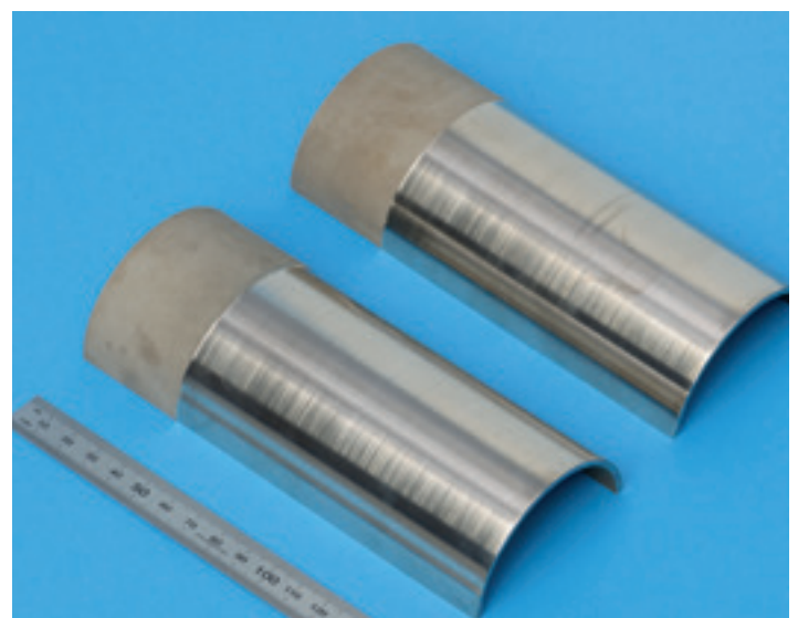
Cold spray formed Ti-6Al-4V half shells made as part of a recent TWI funded research project
