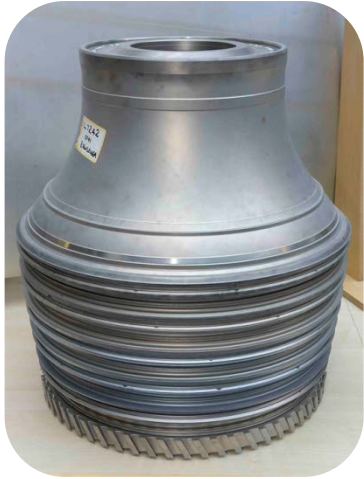
5 EB welds in a turbine drum
