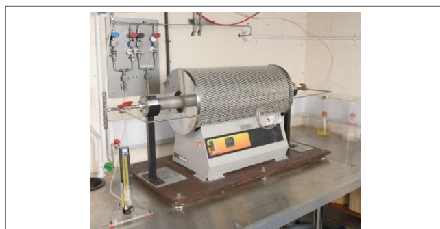
High temperature corrosion cell, accommodating 310 stainless steel test vessel. Safety shielding is not shown in this photograph.
