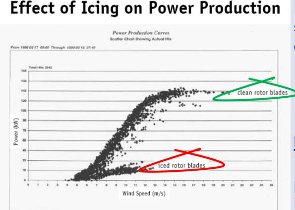
Fouling can cause significant loss of efficiency
