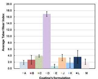
**Coating's formulation Fig.1**: Graphical representation of the Average Taber wear index for each coating formulation, and the deviation.
