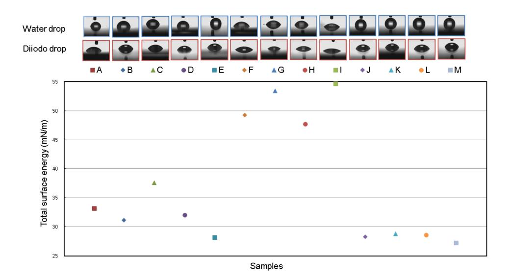
Fig.3: Total surface energy measured for each coating and pictures of the drop of water and diiodo methane which lead to the contact angle measurement
