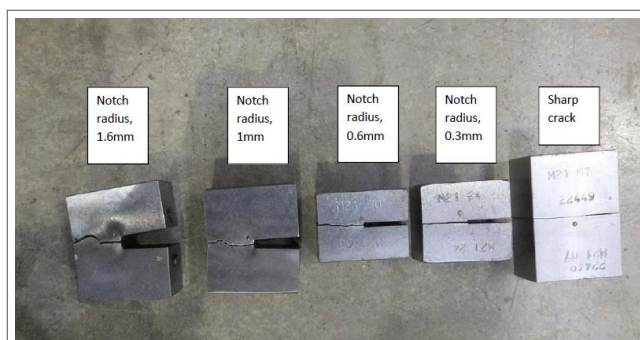
Fracture path of specimens containing different notch radii
