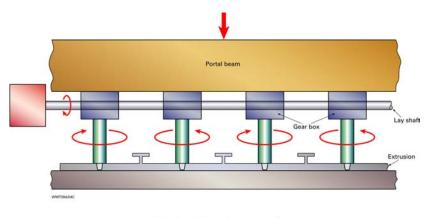
Multi-head friction stir welding machine.
