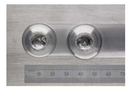
Fig 7. Tandem Twin-stir<sup>™</sup> lead and follow exit holes
