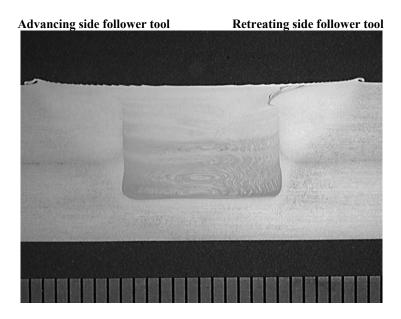
Fig 8. Macrosection of Tandem Twin-stir<sup>™</sup> lap weld in 6 mm thick 6082-T6 aluminium alloy
