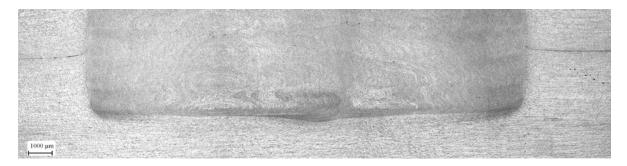
Fig 9. Montage of macrosections taken from the 'common weld region' of a Staggered Twin-stir<sup>™</sup> weld
