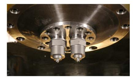
**Fig 5.** Twin-stir<sup>™</sup> prototype head assembly
