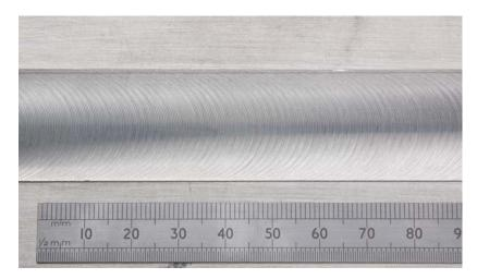
Fig 6. Surface appearance of a typical Tandem Twin-stir<sup>™</sup> weld made in 6083-T6 aluminium alloy
